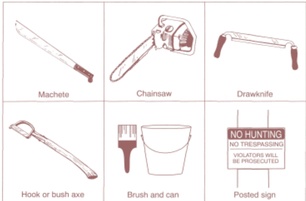
Figure 3. Tools for line marking include the machete, chainsaw, drawknife, hook or bush axe, brush and can, paint brush, and posted signs.
